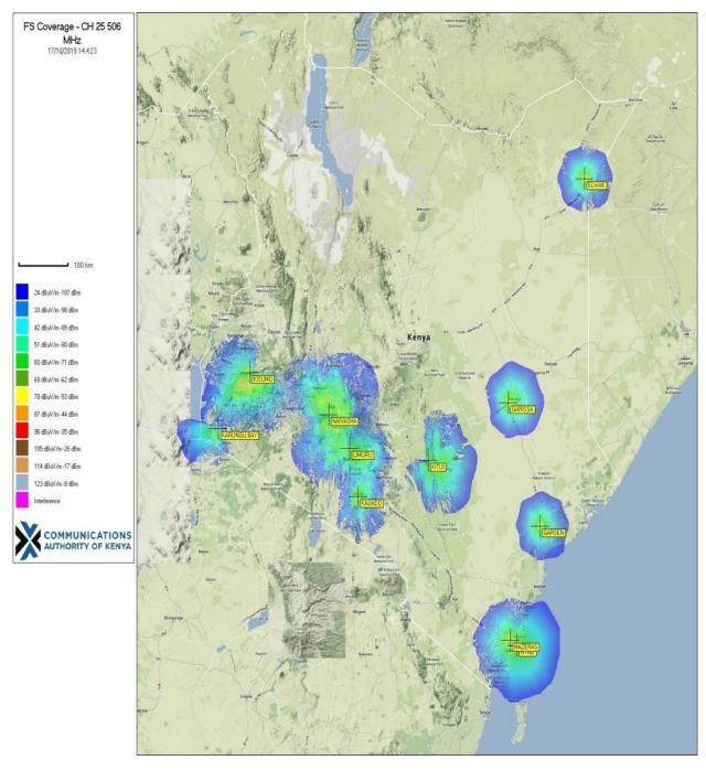
Figure 7.3: Active DTT Transmissions on CH 25 spectrum and available TVWS
