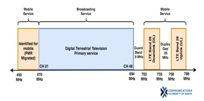
Figure 7.1: Illustration of UHF band Coexistence of Services
