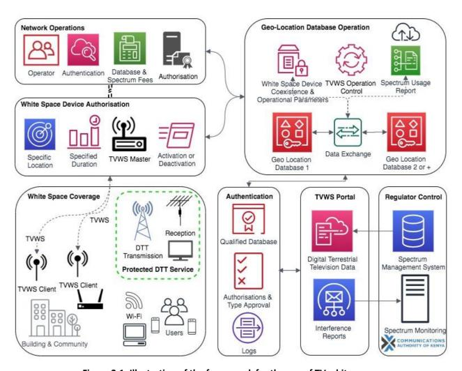
Figure 3.1: Illustration of the framework for the use of TV white spaces
