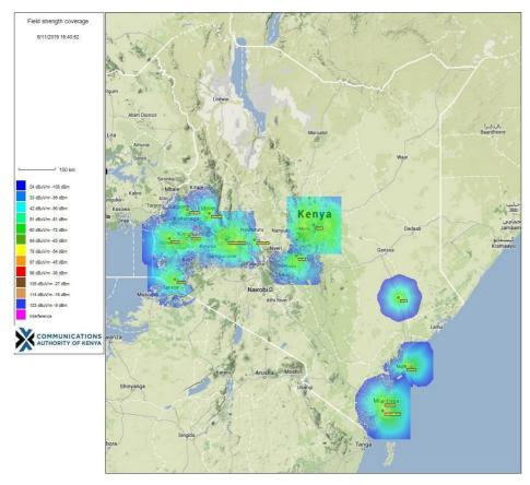
Figure 7.2: Active DTT Transmissions on CH 34 spectrum and available TVWS
