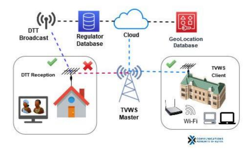
Figure 2.1: Simple diagram of TV White Space Network
