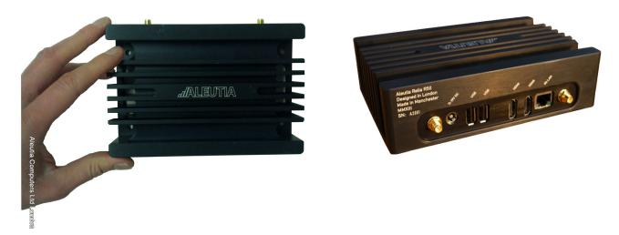
Wall Mountable Industrial High Performance PC Core i3217U CPU (4 x 1.8GHz)
